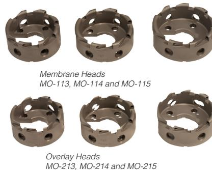
Membrane and Overlay removal heads fit over the tube O.D. and remove the membrane from between boiler waterwall tubes. Additionally, Overlay Heads remove cladding and weld overlay from the tube O.D.
