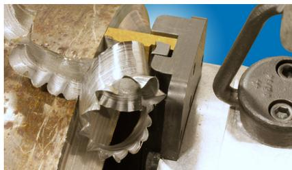
The EscoLock blade lock system and double threaded lock screw hold the blade securely in place to produce a thick chip that helps prolong blade life by transferring the heat to the chip and away from the Cutter Blade.
