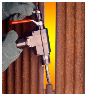
Only 1.5" wide for single boiler tube beveling
