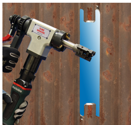
The Tube Weasel is 2.75" wide and can bevel a single tube in a boiler tube waterwall for Dutchman repair.
