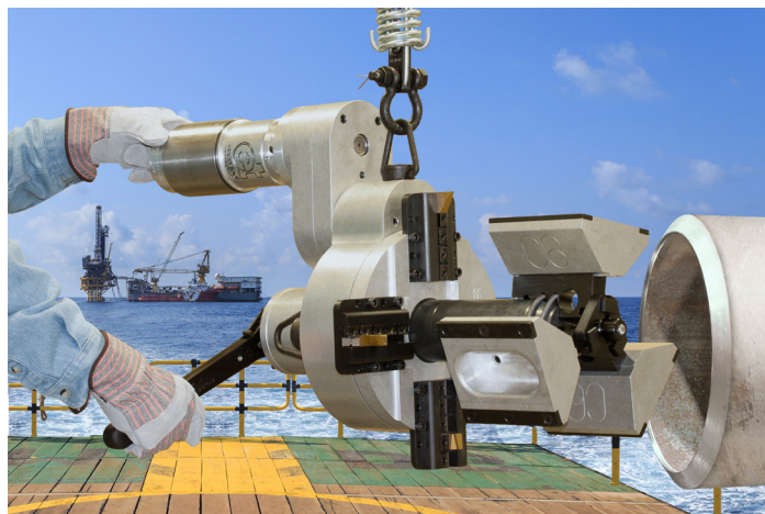
The clamping system of the Commander MILLHOG® Model C-314 pipe beveling machine has six contact points that minimize vibration for chatter free bevels on both thin and heavy wall pipe.
