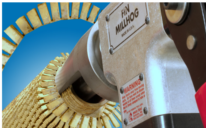
Removes spirally wound fin from tube O.D. The patented cutter requires no cutting fluids and can be resharpened.
