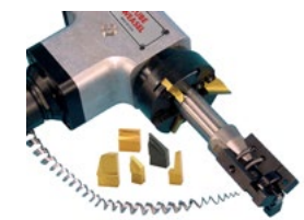
Cutterheads hold 3 Cutter Blades for bevel, face and bore simultaneously 2.75" for use with 0.75" Mandrel 2.75" for use with 1.25" Mandrel 3.0" for use with 1.25" Mandrel
