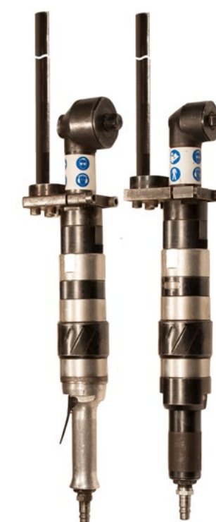
Lever and roll Throttle Torque Control Rolling Motors accurately govern tube expansion and stop automatically when the tube is joined to the boiler tube sheet.
