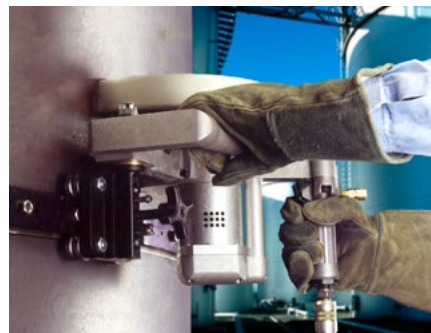
Scoring concrete pilings for height trimming. Concrete Cut-Off Blades are available in Diameters of up to 14".
